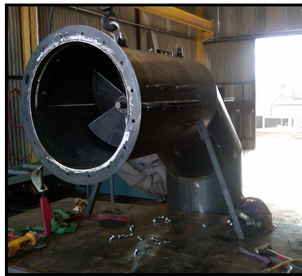
Turbines like this one fabricated by Elephant Butte Irrigation District (NEW MEXICO) can be inexpensively constructed and installed in existing irrigation canal systems.
